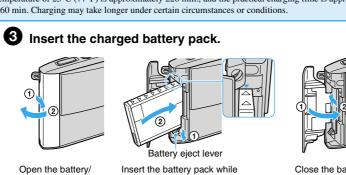
pressing the battery eject level
