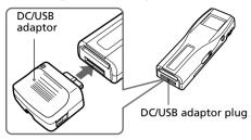
**2** Connect the AC power adaptor to the DC IN 5.5V jack of the DC/USB adaptor and to the wall outlet.
