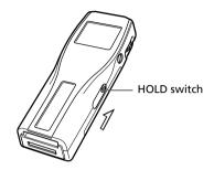
Slide the HOLD switch in the direction of the arrow.
