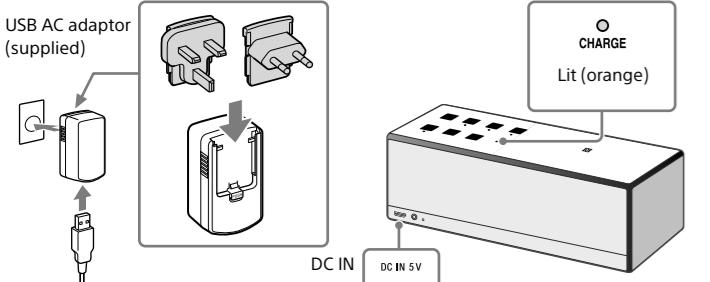
Charging starts when the unit is connected to an AC outlet via the USB AC adaptor, and the CHARGE indicator lights up orange. Charging is completed in about five hours and the indicator goes off.
