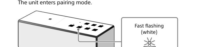
4 Perform the pairing procedure on the BLUETOOTH device to detect this unit.
