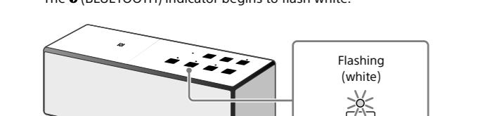
When you use the BLUETOOTH function for the first time, and when you only press the 0 (BLUETOOTH) - PAIRING button, the 0 (BLUETOOTH) indicator will begin to flash white quickly and the unit enters pairing mode automatically.
