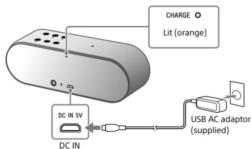
Charging starts when the unit that is turned off is connected to an AC outlet via the supplied USB AC adaptor, and the CHARGE indicator lights up in orange. Charging is completed in about 3 hours and the indicator goes off.
